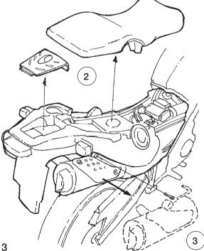
Loosen the screw of the right silencer bracket and remove the right silencer just by pulling it outwards.
