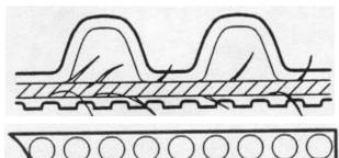
4) Chamfered edge (viewed as a cross section of the toothed drive belt).
