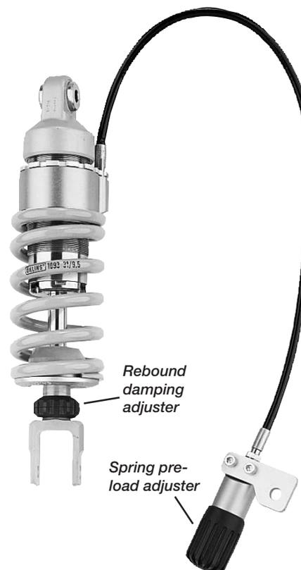
The adjusters have a normal right hand thread. Turn the damping adjusters clockwise to fully closed (pos. zero [0]). Turn counter clockwise to open and count the clicks until you reach the recommended number of clicks. See Setup data at last page.
