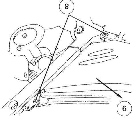
Lift the rear unit backwards, upwards and remove it from the motorcycle.
