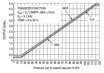
Figure 4. Output versus Absolute Pressure
