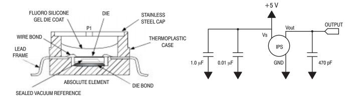
Figure 2. Cross Sectional Diagram SOP (not to scale)
