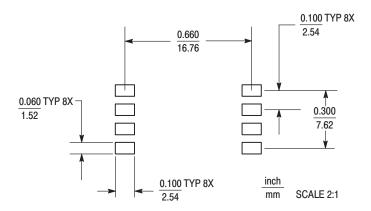
Figure 5. SOP Footprint (Case 482)
