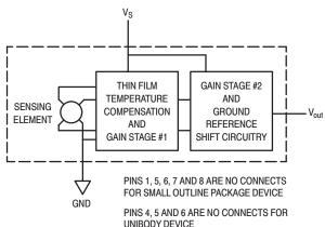
Figure 1. Fully Integrated Pressure Sensor Schematic
